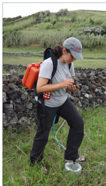
Figure 2 - Measurement of soil CO 2 fluxes with the accumulation chamber method.
