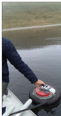
Figure 3 - Measurement of CO 2 fluxes with a floating device.
