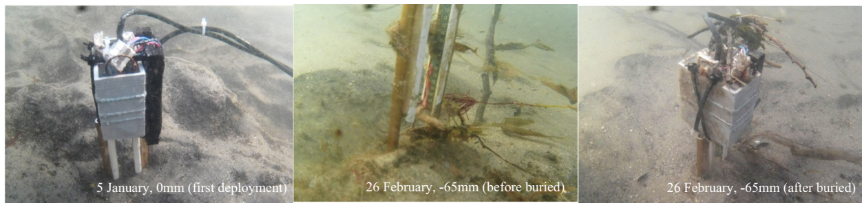
Fig. 7. Underwater photographs of the sediment accumulation sensor at different times of the field test. In the image at left, the moment when the sensor was deployed, with its measure correspondent to 0 mm. In the middle image, the sensor could not provide reliable data anymore since all the 32 optical channels were completely uncovered (26th of February, measure correspondent to -65 mm). In the image at right, also on the 26th of February, the sensor was buried again in the same location (only the vertical position changed), and its measure continued with the value before of -65 mm.
