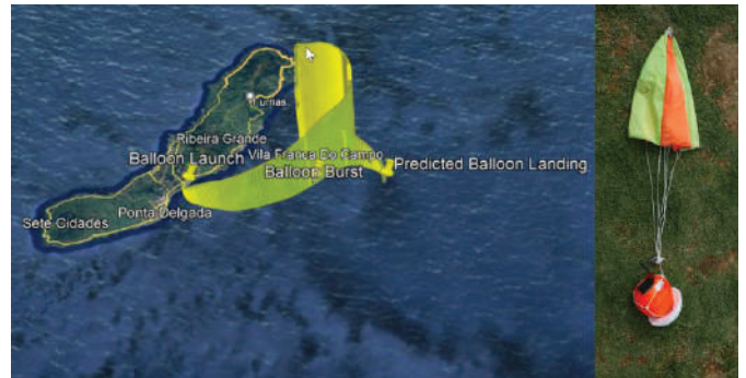
Fig. 9. On the left image is presented the flight simulation of the HAB. On the right image is presented a photograph of the atmospheric probe sprayed orange with a parachute before the launch.
